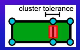
Cluster Tolerance is the distance range in which all vertices and boundaries in a shapefile or feature dataset are considered identical or coincident.
