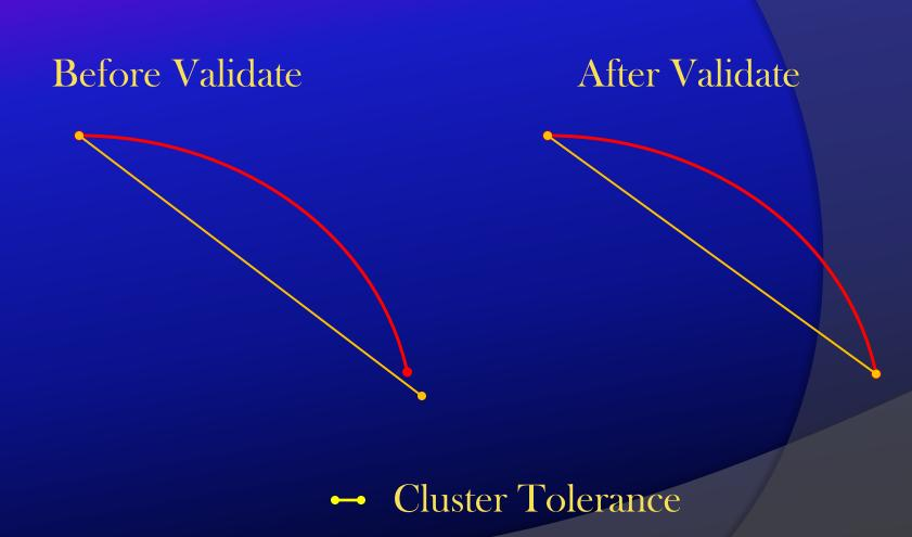
Validate only flags this as an error if the gap or overlap is approx 3 times the Cluster Tolerance
